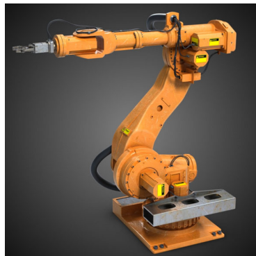
Figure 1.3: A typical serially-connected six-axis robot is a simple open chain.
