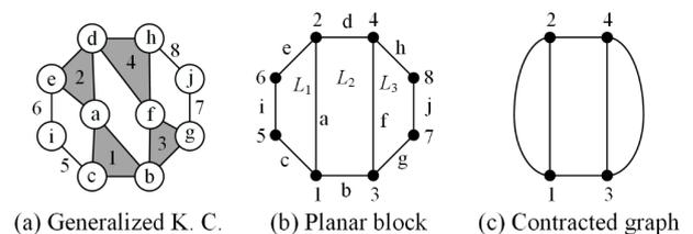
Fig. 1 An (8, 10) generalized kinematic chain, and its corresponding planar block and contracted graph
